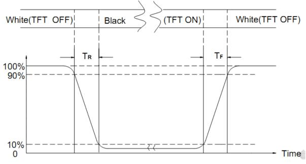
Note (5) Definition of Transmittance (Module is without signal input) Transmittance = Center Luminance of LCD / Center Luminance of Back Light x 100%
